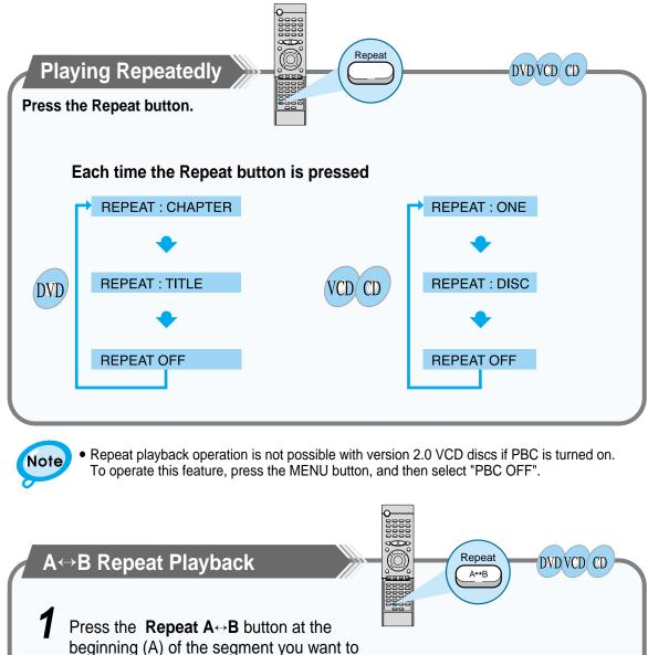
REPEAT : A-Press the **Repeat A**↔**B** button again at the end (B) of the segment you want to REPEAT : A - B • The segment will begin repeating. To return to normal playback REPEAT OFF Press the **Repeat A**↔**B** button again.
